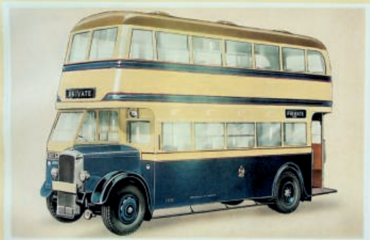
A 54 SEATER HIGHBRIDGE TYPE DOUBLE-DECK Omnibus Body mounted on Gardner chassis and of M.C.W. Patented Metal Construction, built for BIRMINGHAM CITY TRANSPORT.
