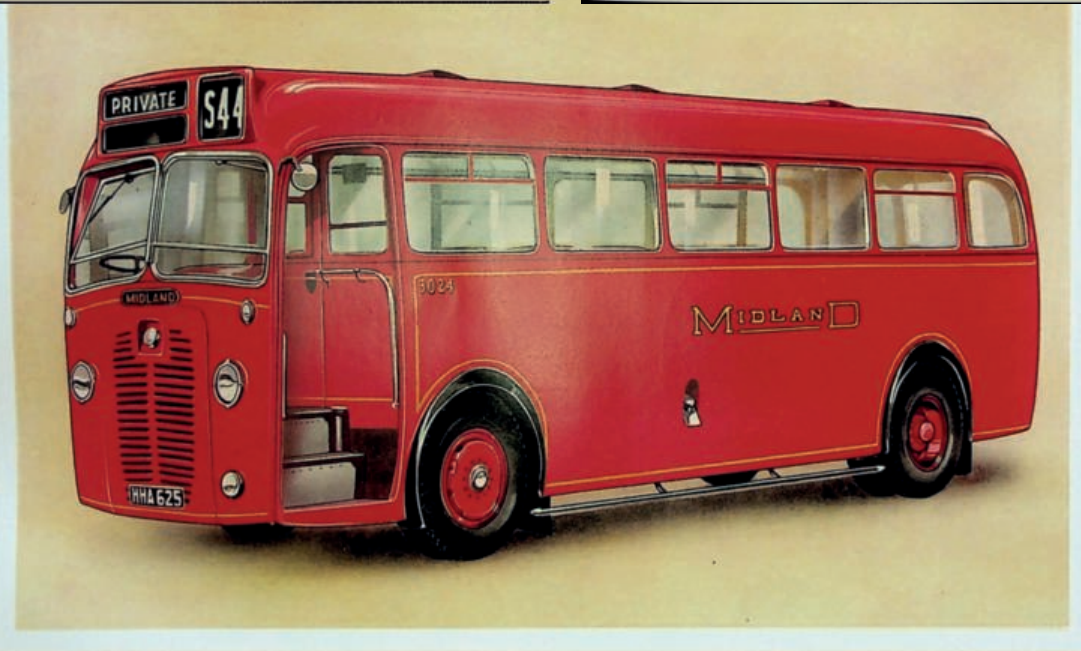
40 SEATER SINGLE-DECK Omnibus Body built for the BIRMINGHAM AND MIDLAND MOTOR OMNIBUS CO. and mounted on operator's own make and type of chassis. This is one of more than 300 similar bodies that
