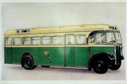
A 46 PASSENGER (24 seated-22 standing) SINGLE-DECK Omnibus Body mounted on A.E.C. "Regal" chassis with rear drop-frame seats for LISBON ELECTRIC TRAMWAYS LTD. The bodies 8' 0"
