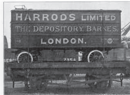
FIG. 4.—Roping a Furniture Van on Wheels over all.
